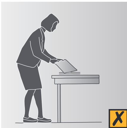
Figure 4.8 Incorrect standing-height bench
