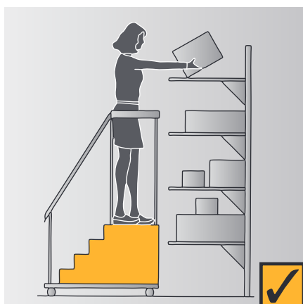
Figure 4.18 Controlling risk of storage at height
